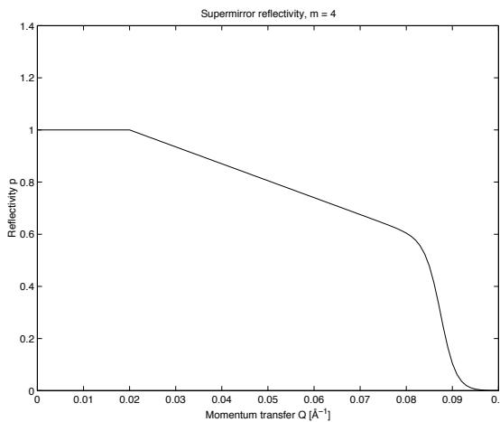
Figure 5.1: A typical reflectivity curve for a supermirror, Eq. (5.2). The used values are
